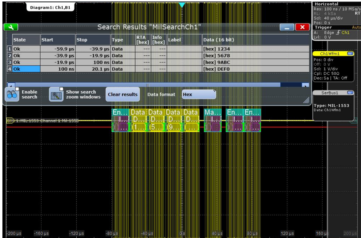
Figure 12-49: Results of a search for all data words (any RTA and any data pattern)
